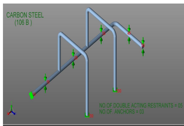
Fig 1.7 CAESAR II routing of Carbon steel material
